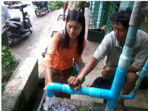
Taking Water Sample for Testing of Lead Content in Drinking Water Source
